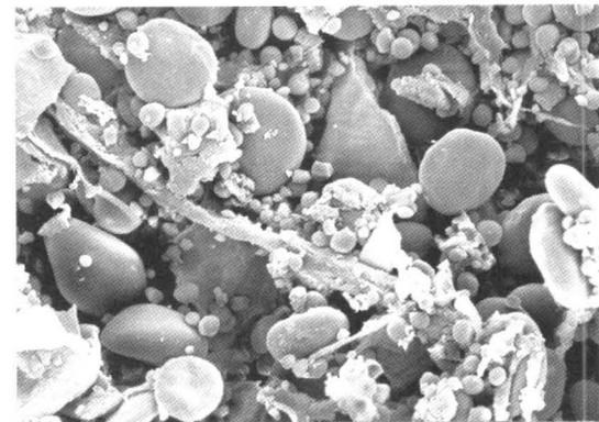
**Fig. 2.** Developed soft wheat dough chemically fixed with 4% glutaraldehyde followed by ethanol dehydration and critical point drying with CO<sub>2</sub>. (2000X).
