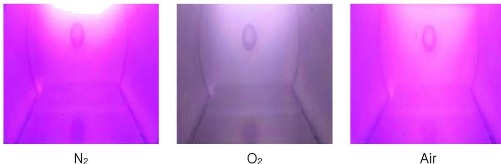
Fig. 2. Appearance of low-pressure plasmas of different gases.
