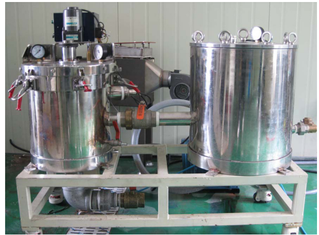
Fig. 2. Photograph of vacuum puffing machine for non-deep fried Yukwa.
