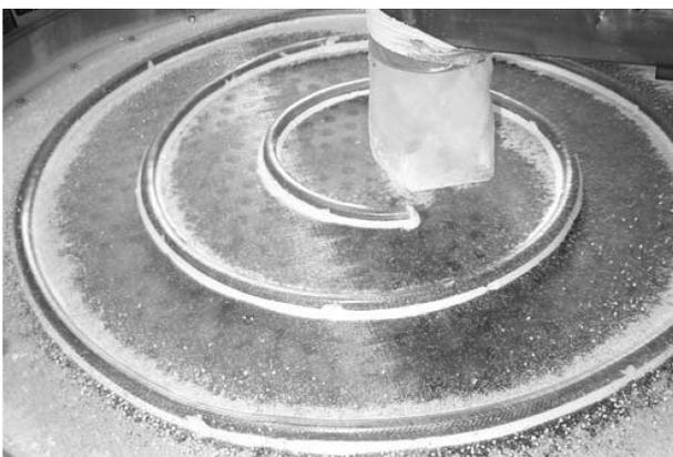
Fig. 6. Photo of screen with spiral blockage.
